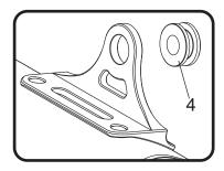
2. Install (No. 5) *ALS-043* aluminum spacers into (No. 4) *Z102*4, rubber grommet as shown.
