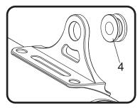
2. Install (No. 5) ALS-043 into (No. 4) Z1024, rubber grommet as shown.
