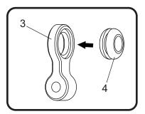
Install (No. 11) ALS-051, aluminum spacer into frame and secure using (No. 5) M8X60H, bolt, (No. 8) 8MMWASHERXL, XL washer, (No. 9) ALS-003, aluminum spacer, and (No. 6) 8MMNUT, flange nut as shown. Do not torque at this time.
