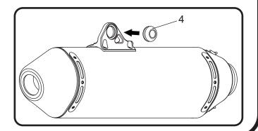
8. Install (No. 10) *ALS-004*, aluminum spacer into (No. 4) *Z1022*, rubber bushing in muffler bracket as shown.
