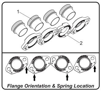
2. Install (No. 3) *13630-404/13630-704*, header onto manifolds by slipping one header leg at a time from one end to the other. Using a rubber mallet, gently tap header legs to make sure header is fully seated onto the manifolds.
