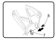
2. Align (No. 7) 13141-RMBKT, muffler bracket adapter to the backside of the right footpeg bracket. Secure using the stock bolt.
