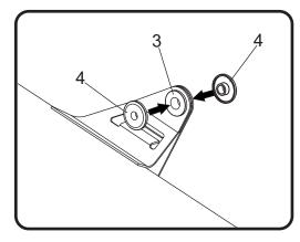
Install (No. 1) 12400BD520-RMA, muffler assembly over the stock header outlet and secure muffler to chassis using (No. 6) M8X55, bolt (No. 7) M8ALCSW-00, countersink washer, and (No. 5) 8X25SPCR, aluminum spacer as shown.
