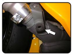
5. Install (No. 6) *M6X1U*, U-Nut onto the heatshield bracket as shown.
