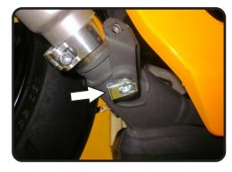
Install (No. 2) 11600-HS, heatshield using (No. 4) M6X10BHS and (No. 5) M6X12BHS, button head screws.
