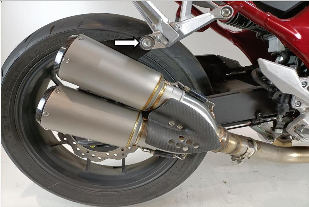
Detail of correct bracket position using stock bolt and nut.
