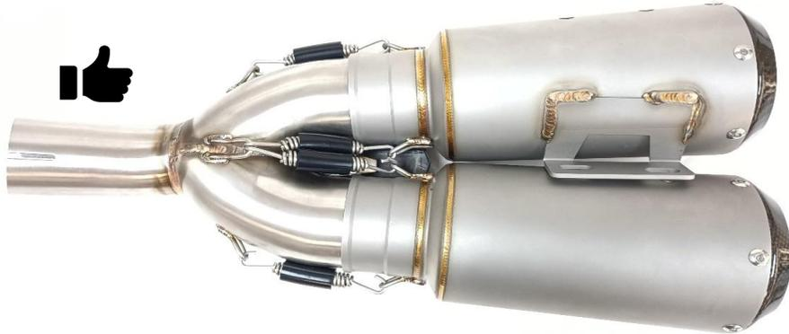
Use 2 x M8x16 screw, 2 x M8 washer & 2 x M8 lock washer from our installation kit to join both mufflers. Both screws must be tighten.
