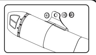
3. Apply supplied anti-seize inside tailpipe inlet joint and spread evenly. Install muffler assembly onto header outlet and align chassis mount and muffler mount. Secure using the stock chassis mount bolt and muffler mount bolt. Do not torque at this time.
