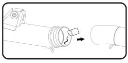
4. Torque header nuts to factory specification and install *RACE-SPX-2*, short exhaust springs between header flange and spring hooks.
