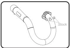
2. Install *Z1024*, rubber grommet into muffler bracket and install *ALS-038*, spacer and *ALS-039*, spacer cap as shown.
