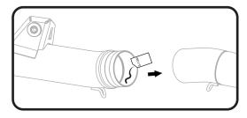
4. Torque header nuts to factory specification and install *RACE-SPX-2*, short exhaust springs between header flange and spring hooks.
