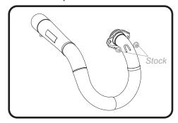
2. Install *Z1024*, rubber grommet into muffler bracket and install *ALS-038*, spacer and *ALS-039*, spacer cap as shown.
