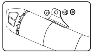
Apply supplied anti-seize inside tailpipe inlet joint and spread evenly. Install muffler assembly onto header outlet and align chassis mount and muffler mount. Secure using the stock chassis mount bolt and muffler mount bolt. Do not torque at this time.
